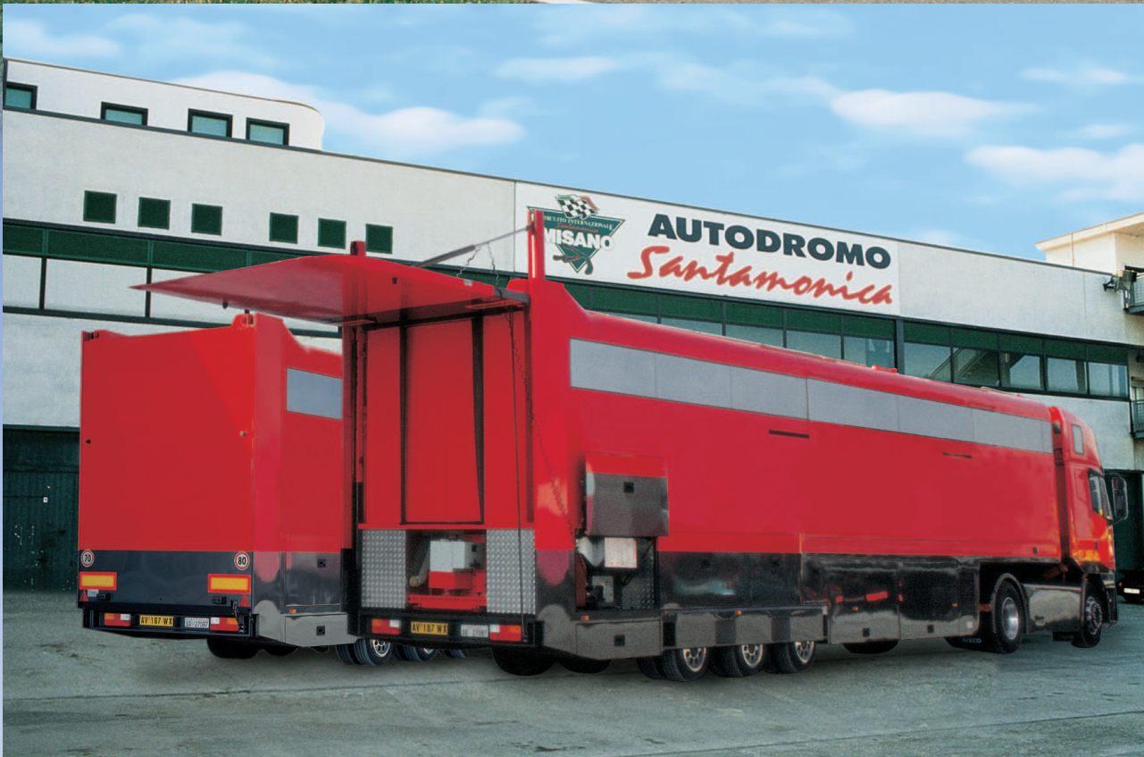
Piattaforma mod. RACING 1500 Speciale, installata su van Scuderia Ferrari Marlboro F1. Special "Racing" platform installed on a Ferrari Marlboro F1 Team van.
